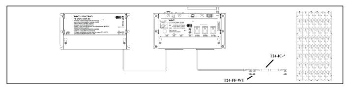
5. To extend the cable length between Wireless DMX LED Controller cable or a wiring box to a PIXELS sections, (if needed), In Wall Rated Extension cable (T24-EX3-\*) can be used to join between sections by soldering as shown in FIG. 7. Wire color connection is shown in the Table 1.
