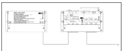
Mounting 24VDC Class 2 remote power supply and WAC Wireless DMX LED
